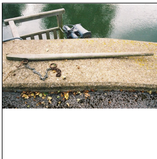
THA/MT/ E/2: Lever tool for lifting wooden paddles out when swollen.
